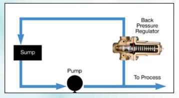
SERIES BS - **CONSTANT PUMP DISCHARGE PRESSURE**By using a simple spring loaded back pressure regulator, constant pump discharge pressure can be generated regardless of demand.
