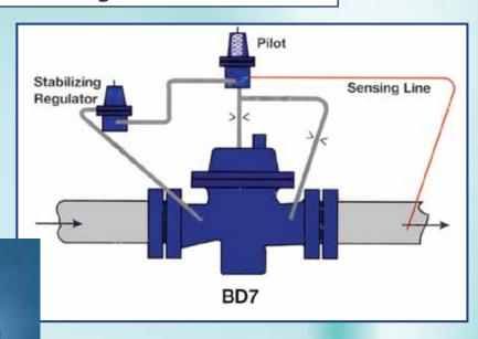
Typical pilot actuated dome loaded regulator for regulator accuracies of  $\pm$  0.1-0.2 psig.
